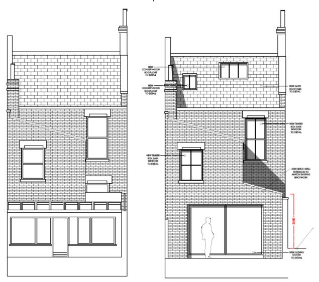
Figure 2: existing (left) and proposed (right) rear elevation
